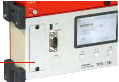
Switching box/TML-NET driving board (Factory-installed option)
