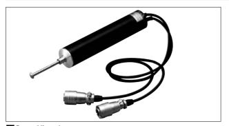
The CDP-D displacement transducer is the CDP displacement transducer with dual isolated I/O ports. For example, one set of input and output cables can be connected to an analog measuring instrument and the other set to a digital measuring instrument. With two different types of measuring equipment connected to this transducer, simultaneous measurements can be made without interference.
